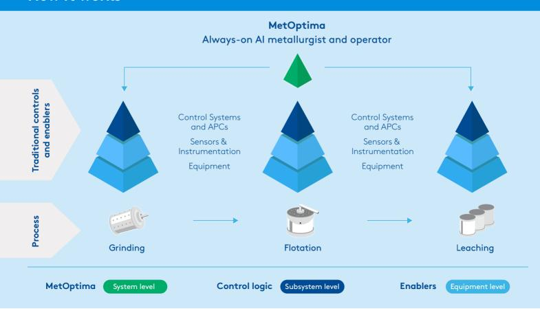
MetOptima leverages aggregated plant and sensor data through the client adapter and applies our suite of advanced analytical and predictive models to the data to generate recommendations every few hours, which the shift operator either accepts or rejects via a user-friendly web app.
